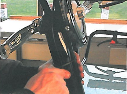
7.b mounting gear cable to plastic strip
