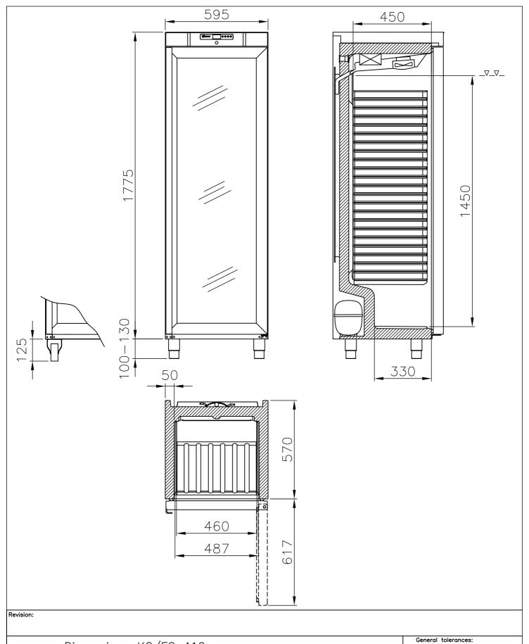
Description: Dimensions KG/FG 410 ISO 2768-1 (v) A format 11/09/09 Drawing no.: Date: Sheet no.: Rev. (TRAW) JABP Name: 000 4 © Gram Commercial A/S 1/15 Scale DENMARK
