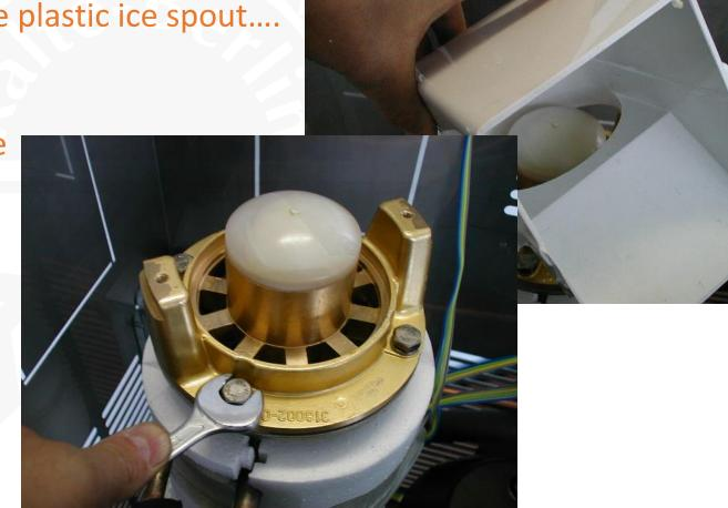
With a couple of screwdrivers rise up a little bit the ice breaker and auger assembly then ....
