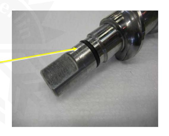
Slide off from the bottom of the auger the upper half of the water seal.
