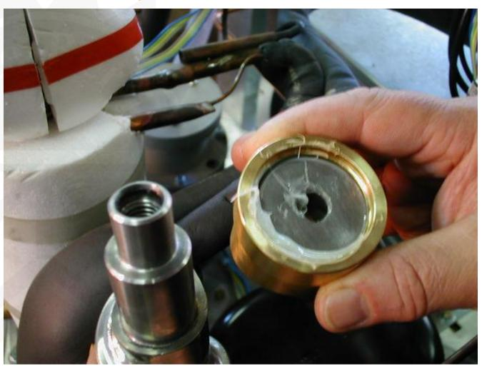
Clean away the old grease from the interior of the ice breaker and inspect the conditions of the top bearing .....
