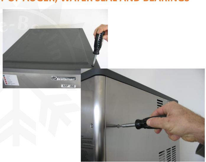
Unloose the four screws holding the metal bracket and remove it from the frame of the machine
